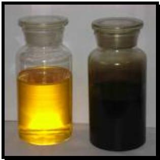
On the left is a picture of new motor oil. On the right is a picture of old motor oil. The difference is startling and easy for anyone to recognize...even a novice.
